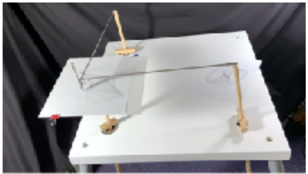
3 pendulum rotary harmonograph
