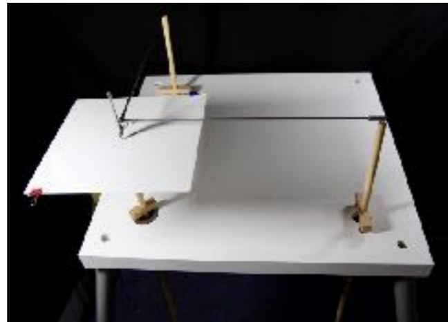
rotary harmonograph (3 pendulum)
